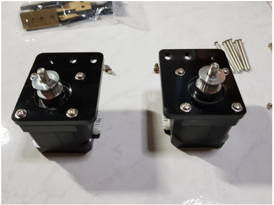
Note the position of the white connectors, they have to be facing exactly as pictured.
